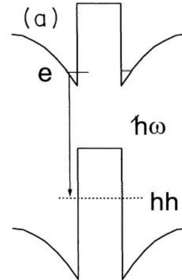
At higher powers an excess of holes and electrons are created at the interface between the two semiconductors. For Type II, the spatial separation of carriers in CB and VB will induce an electric field which bends the energy level and increases the gap.
